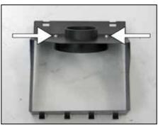
9. Install the K&N<sup>®</sup> filter adapter into the heat shield as shown and secure with the provided hardware.
