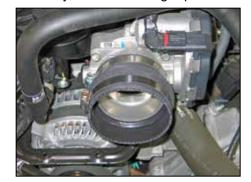
16. Install the provided silicone hose (08699) onto the throttle body and secure with the provided hose clamp.
