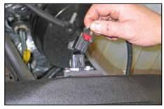
24. Connect the provided mass air sensor extension harness into the factory harness connection, and then connect the open end to the mass air senor electrical connector.
