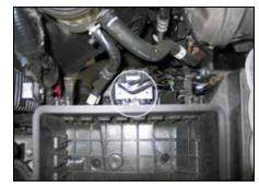
8. Remove the center upper air box retaining clip from the lower air box.
