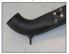
21. Install the provided crank case vent fitting into the  $K\&N^{\circ}$  intake tube as shown.
