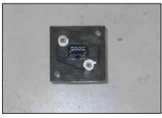
19. Install the mass air sensor into the mass air adapter and secure with the provided screws.
