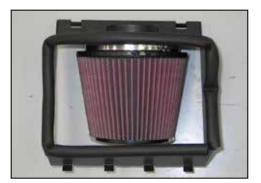
13. Install the K&N<sup>®</sup> air filter onto the filter adapter and secure with the provided hose clamp. NOTE: Drycharger<sup>®</sup> air filter wrap; part # RC-5173DK is available to purchase separately. To learn more about Drycharger<sup>®</sup> filter wraps or look up color availability please visit http://www.knfilters.com<sup>®</sup>.
