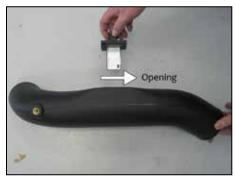
20. Install the mass air sensor assembly into the K&N<sup>®</sup> intake tube as shown.
