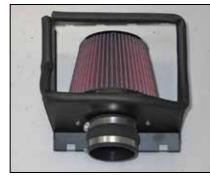
14. Install the provided silicone hose (08699) onto the filter adapter as shown and secure with the provided hose clamp.
