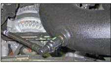
23. Rotate the crank case vent coupler so that it lines up with the fitting installed in the K&N<sup>®</sup> intake tube, then connect the coupler to the fitting.
