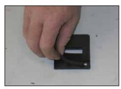
18. Install the provided gasket onto the K&N<sup>®</sup> mass air sensor adapter.
