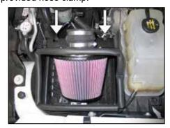
15. Install the completed heat shield / air filter assembly onto the lower air box and secure with the two factory air box retaining clips.
