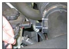
2. Release the red locking tab and then disconnect the mass air sensor electrical connection.
